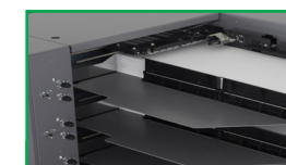
8-belt air suction feed system and Air Management System ensure reliable feeding.
