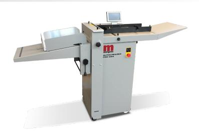
All settings and adjustments are made using the new SmartScreen and as only symbols are used, operation couldn't be simpler. An alpha-numeric memory allows up to 50 jobs to be stored and named as you choose. This makes job recall much easier as you can use your own job name and numbers for storage.
