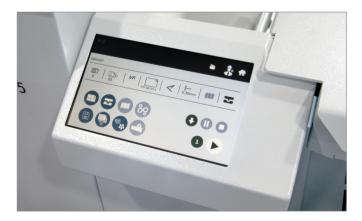
Up to 8500 A4 sheets per hour can be produced with the crease position accurate to +/- 0.004" with a maximum sheet size of 15.16" x 27.5". Up to 16 creases per sheet can be placed as close as 0.04" apart.
